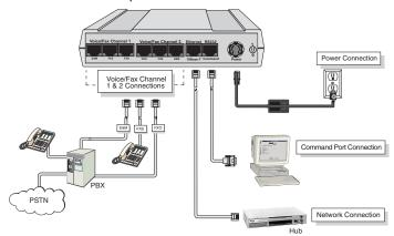
Figure 3. Cable Connections
